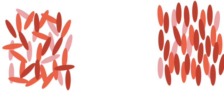
(a) Schematic of the isotropic liquid phase of a system of elongated molecules. (b) Schematic of the nematic liquid phase of a system of elongated molecules. This phase has uniaxial ordering.
